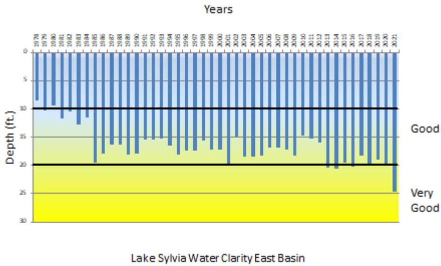
Figure 2. Average Secchi disk measurements from 1974 thru 2021.
